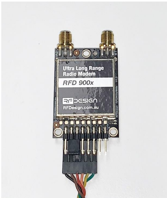
Figure 8 - Modem connected to FTDI cable (pins 1,3,5,7,9, and 11) to enable serial communications, and jumper connected to pins 4 and 6.
